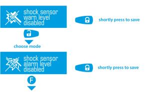
For a prompt remote adjusting of the shock sensor security zones, select «ADJUSTING SHOCK SENSOR WARN LVL» or «ADJUSTING SHOCK SENSOR ALARM LVL» submenu by short presses of [] button. Sensor sensitivity can be set with short presses of and buttons.
