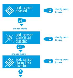
For a prompt remote adjusting of the additional sensor security zones, select «ADJUSTING ADD SENSOR WARN LVL» or «ADJUSTING ADD SENSOR ALARM LVL» submenu by short presses of button. Sensor sensitivity can be set with short presses of and button.
