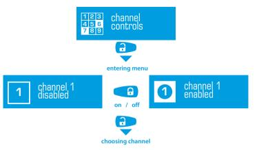
• shortly press 🔒 button to switch between channels 2,3 and 4.
